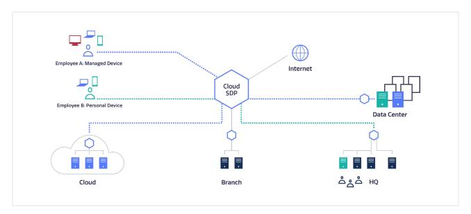
Unlike VPNs' overly permissive access, SDPs enforce restricted, identify-based access. Here, we see that Employee A can access one application in the data center and one in the cloud, while Employee B can only access a single application at HQ.
