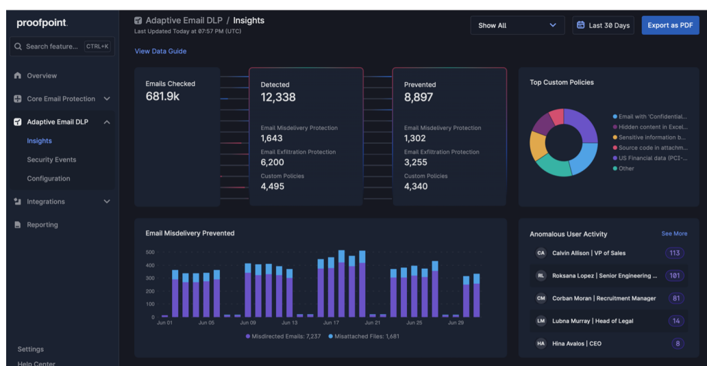
Figure 4: The Adaptive Email DLP insights dashboard shows statistics about email data loss detection and prevention. This includes metrics about email misdelivery, email exfiltration, custom policies applied, and users with the most anomalous behavior.
